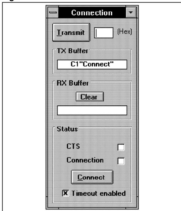
The *Connection Window* is made up of a *Transmit* button and three frames : *TX Buffer*, *RX Buffer* and *Status*.
